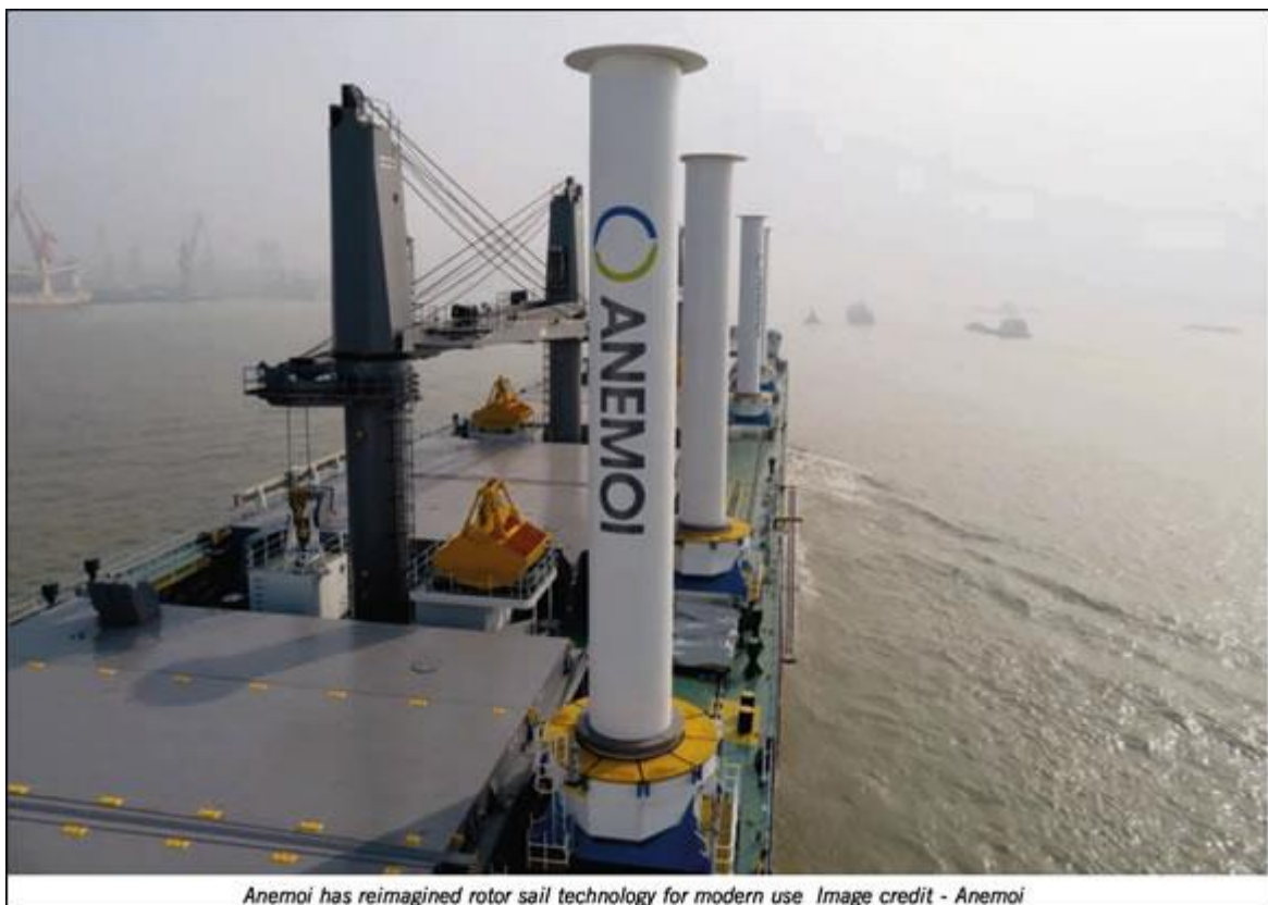
Anemoi has reimagined rotor sail technology for modern use Image credit - Anemoi
