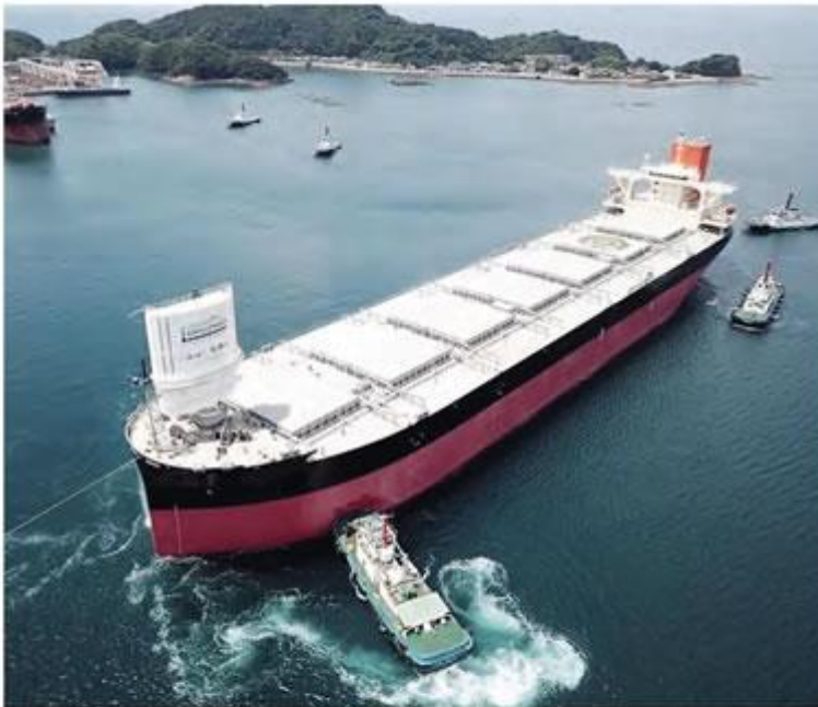
The Shofu Maru (2022) is the first bulk carrier with a Wind Challenger hard sail. The Wind Challenger Project was developed by the Tokyo University in cooperation with Mitsui O.S.K. Lines (MOL) en Oshima-shipbuilding. The Shofu Maru is testing the system with a single mast. Next project can be a bulk carrier that will be delivered in 2024 and maybe gets extra rotor sails from Anemai Marine Technologies.
